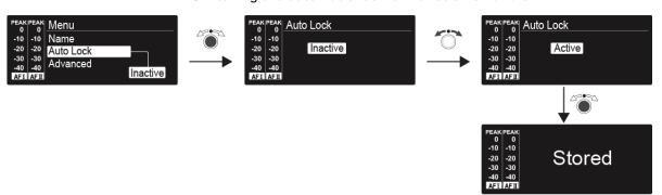
This lock prevents the transmitter from being unintentionally switched off and also prevents any unintentional changes to the transmitter's configuration. In the standard display, the lock icon shows whether the lock-off function is currently switched on.
