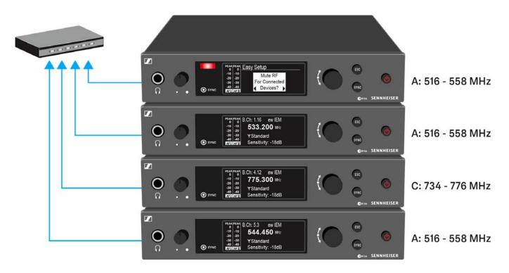
▶ Press the jog dial to confirm the message and deactivate the radio signal for all connected transmitters.
