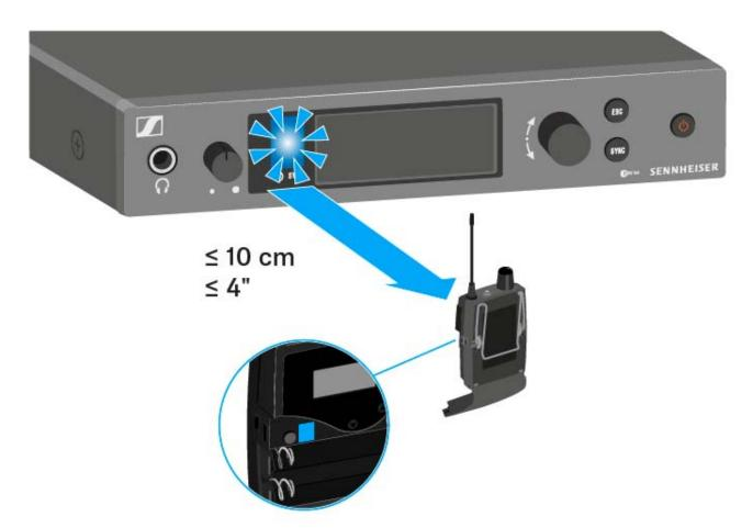
The parameters are transferred to the receiver. The blue LED blinks during transmission.
