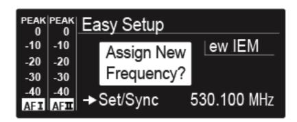
▶ Press the jog dial (SET) on the particular transmitter to save your selected frequency and synchronize it with the corresponding receiver at a later point (see "Synchronizing devices").
