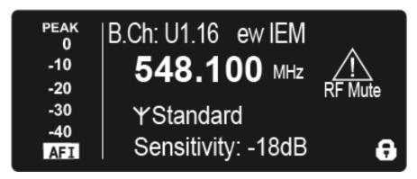
In Mono mode, you have to deactivate the pilot tone evaluation on your EK IEM G4 receiver. This is the only way to ensure that your receivers will transmit the same signal on channel I and channel II.
