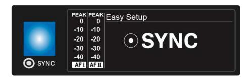
▶ Perform a frequency preset scan with your EK IEM G4 mobile receiver (see "Easy Setup menu item") and select a frequency bank with sufficient unused frequencies.
