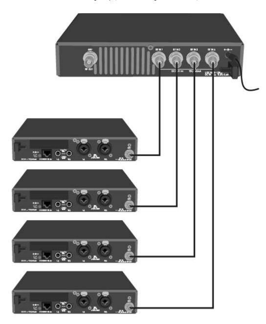
The SR IEM G4 and SR 300 IEM G3 transmitters are supplied with voltage via the RF IN input sockets of the AC 41.
