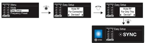
The **Easy Setup Sync** function is needed to perform a frequency scan using the receiver and for automatic multi-channel frequency setup.
