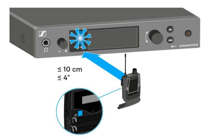
The next unused frequency preset is transferred from the receiver to the transmitter.
