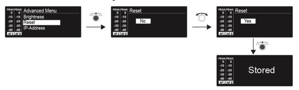
When you reset the transmitter, only the selected settings of the pilot tone and the **U1** to **U6** frequency banks are retained.
